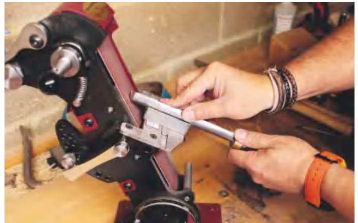
▲ The 'V' block cradle allows roughing gouges to be easily worked
